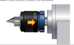
3.再將鎖緊螺帽以手旋轉貼合尾座軸套端面。 please turn the draw-off nut close up the face of tailstock.
